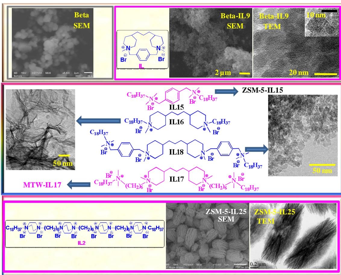
Scheme 1. Synthesis of ordered and disordered zeolites of different framework structures.
